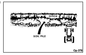
Leave dirt which drifts over side of bucket for final cleanup.
